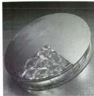
18" diameter, 60% lightweighted mirror blank
